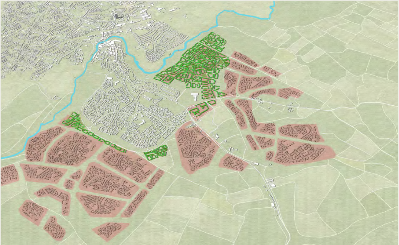
The gentle density masterplan (in green) takes up two-thirds less land on the edge of Chippenham than the original road-led masterplan (in red)
